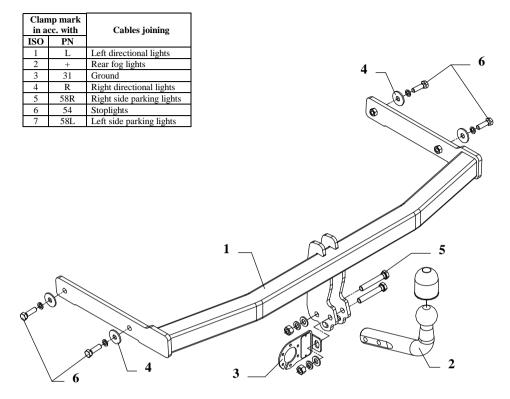
This towbar is designed to assembly in following cars: **SEAT TOLEDO, 4 doors,** produced since 05.1998 till 2004, catalogue no. **SC19** and is prepared to tow trailers max total weight **1600 kg** and max vertical load **75 kg**.
